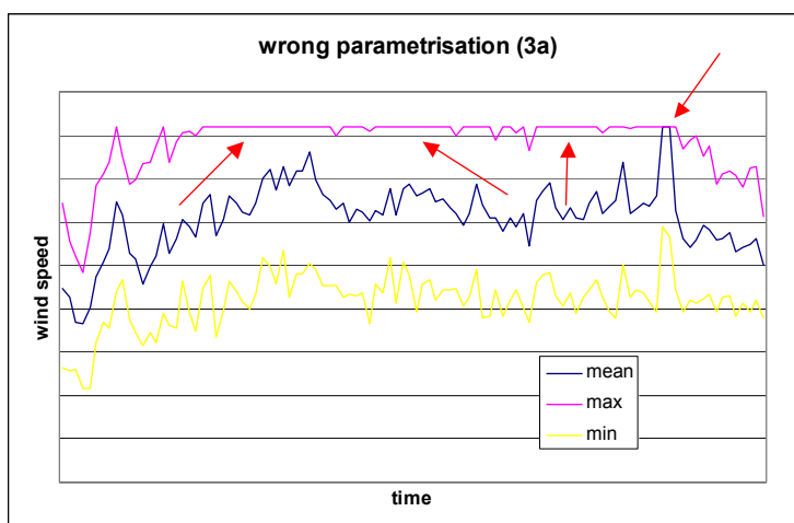
Figure 2: Consequence of wrong parametrisation of data logger
